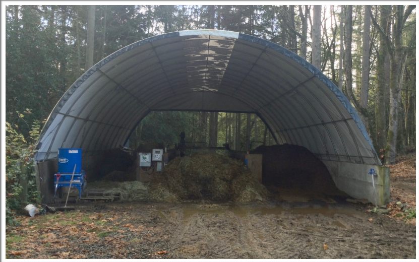
Auger Composting System by Green Mountain Industries. Approximately 30'X70'. Can aerobically produce up to 500 yards of compost a month. Uses 50% less space and can produce compost nearly 3 times faster than machine turning. This unit in use at Hey Day Farm.
