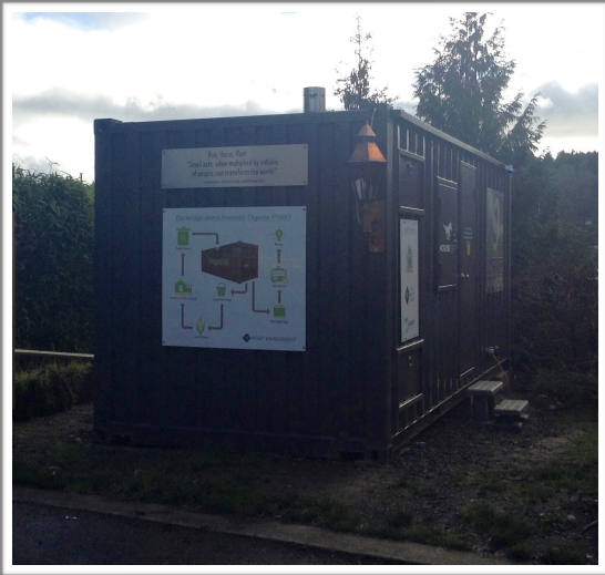
Auger Composting System by Green Mountain Industries. Approximately 30'X70'. Can aerobically produce up to 500 yards of compost a month. Uses 50% less space and can produce compost nearly 3 times faster than machine turning. This unit in use at Hey Day Farm.
